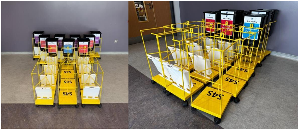
Figure 1: Bespoke Bin Collection System, Fabrication and cart modifications.
